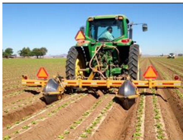
Figure 3.6d Use of Bolas to Reduce Resistance to Water Flow in Furrows
